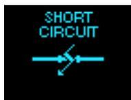
Non high drain battery or poor contact between the battery and board
